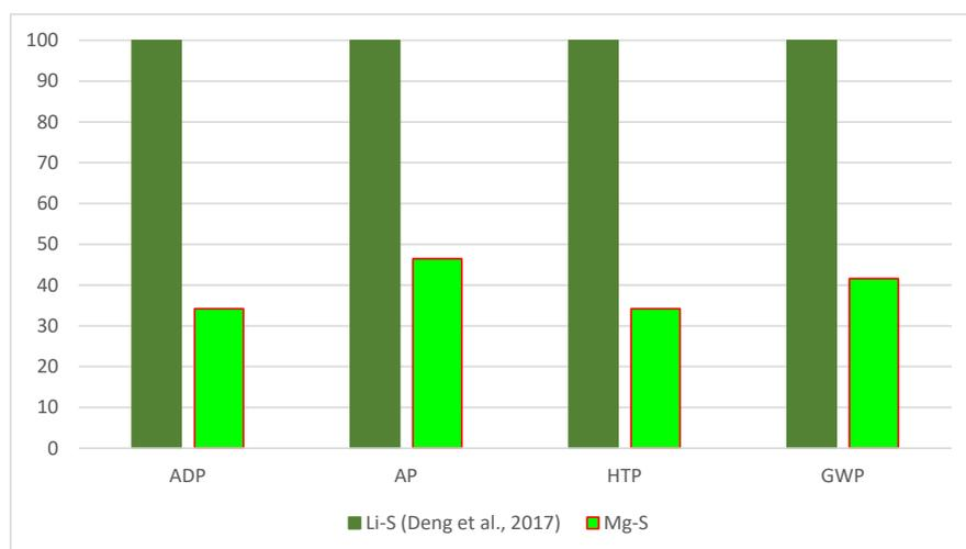
**Figure 19:** Environmental profile of the future Mg-S battery compared to Li-S reference battery. The environmental burden of this future Mg-S battery is supposed to fall from 55 to 65% compared to the selected reference.
