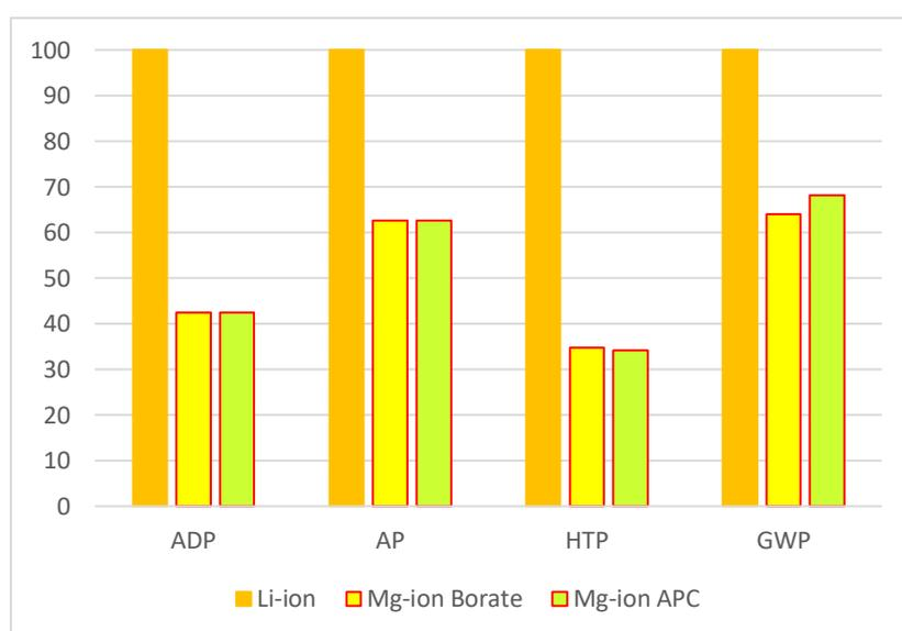
**Figure 17:** Comparison of the environmental profiles of the two future Mg-ion batteries for ADP, AP, HTP and GWP impacts.
