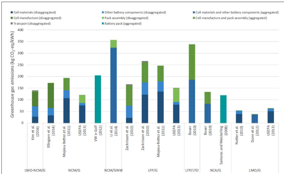
Figure 8: Graphical representation of the LCA results for GWP for different LIB chemistries (Ellingsen et al., 2017).
