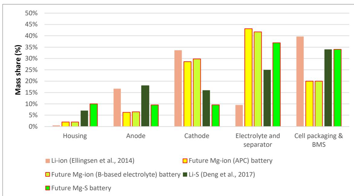
**Figure 14:** Future RMB mass breakdown and comparison to existing battery breakdown (All the sources are referenced in the legend).
