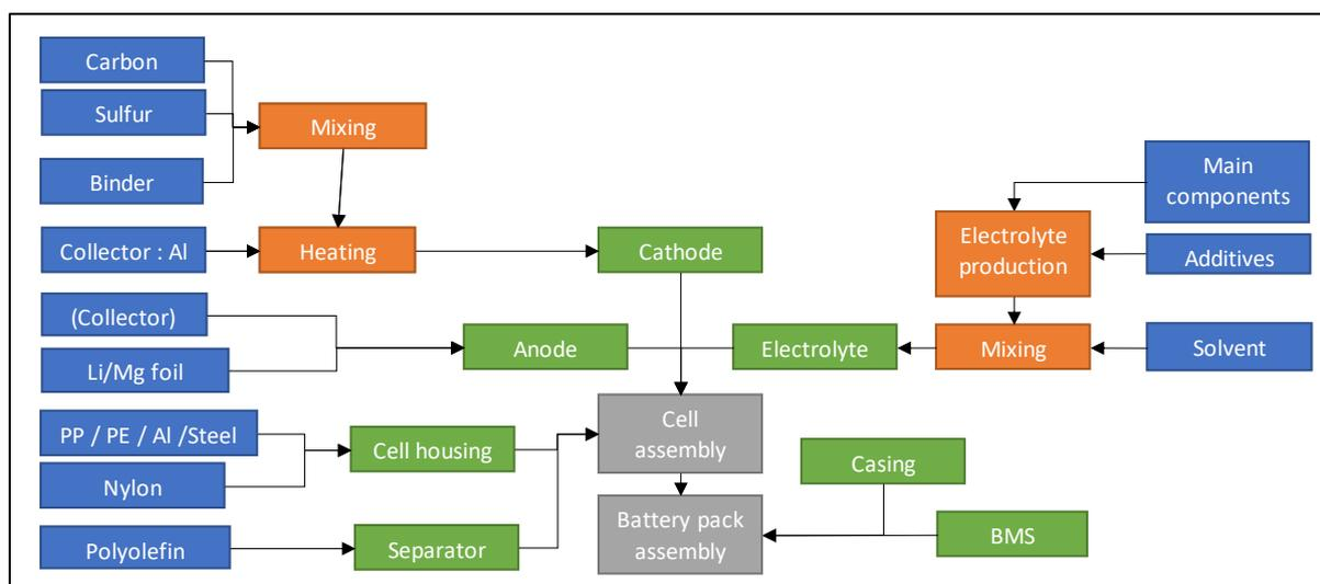
**Figure 4 : Simplified flow chart of the X-S batteries.**
