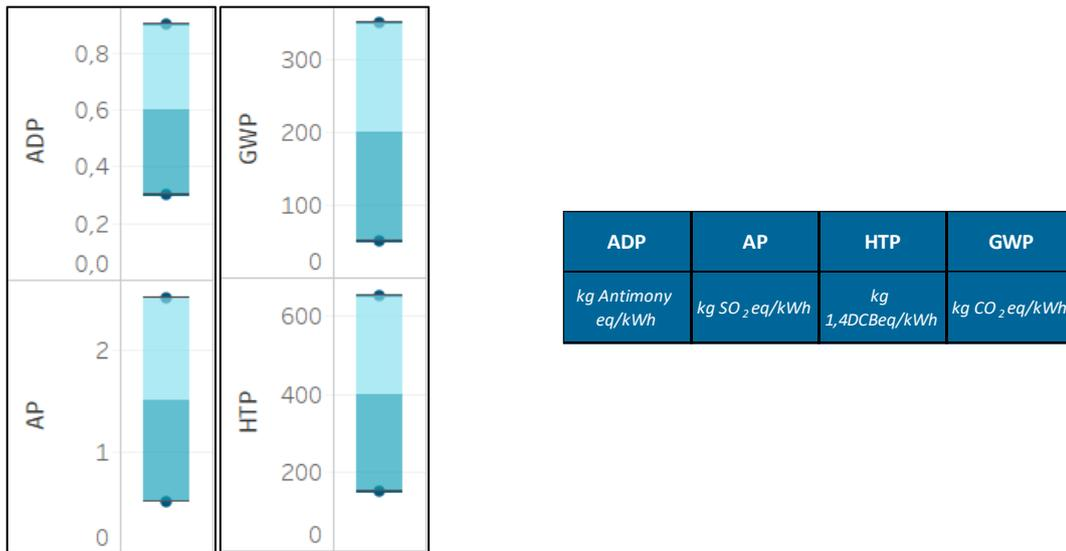
Figure 7: Cradle-to-Gate LIBs LCA impact ranges for the selected impact categories and associated units (Peters et al., 2016).
