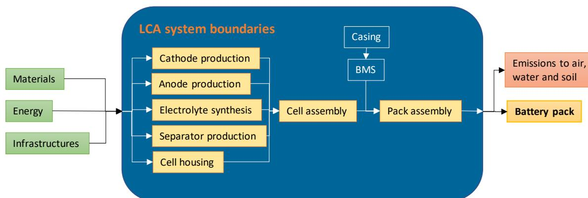
**Figure 3 :** System boundaries schematic description in cradle-to-gate approach.
