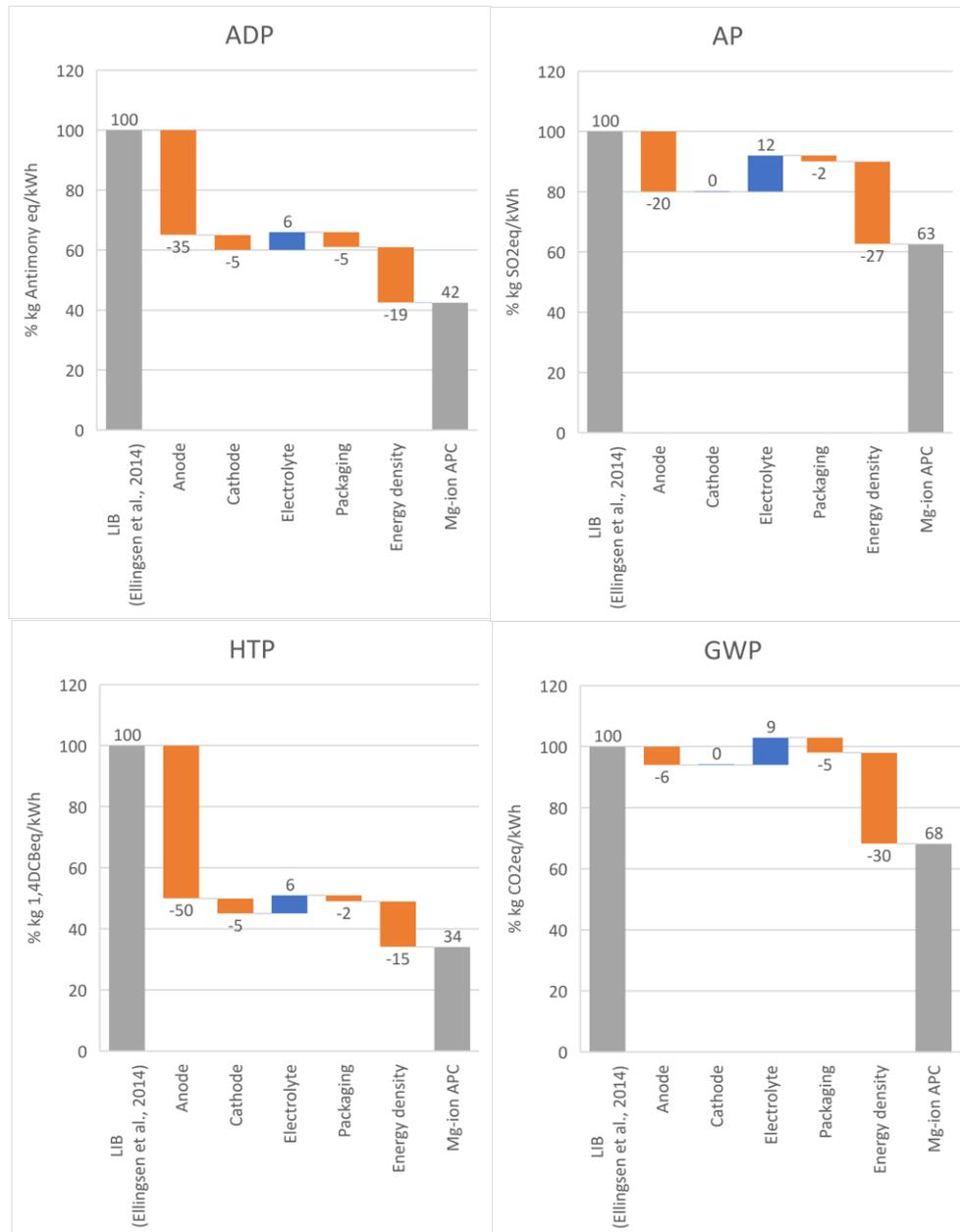
Figure 15: Estimated environmental profile of the future Mg-ion (APC) battery compared with the Li-ion battery from Ellingsen et al. (2014).
