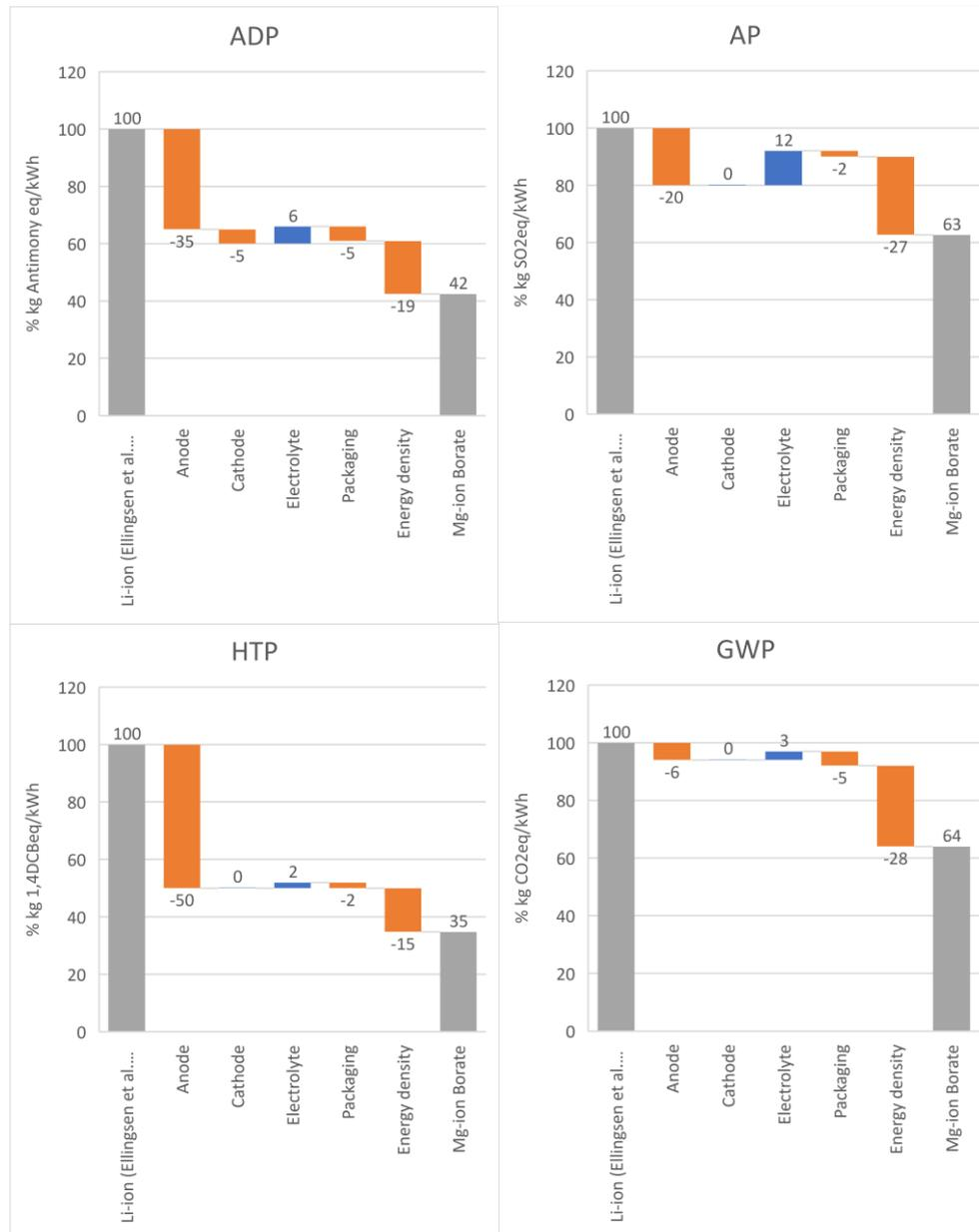
**Figure 16:** Estimated environmental profile of the future Mg-ion (Borate-based electrolyte) battery compared with the Li-ion battery from Ellingsen et al. (2014).
