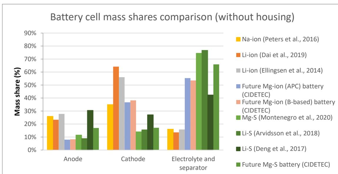
**Figure 10:** Overview of mass breakdowns of different battery cells (all the sources are referenced in the legend).
