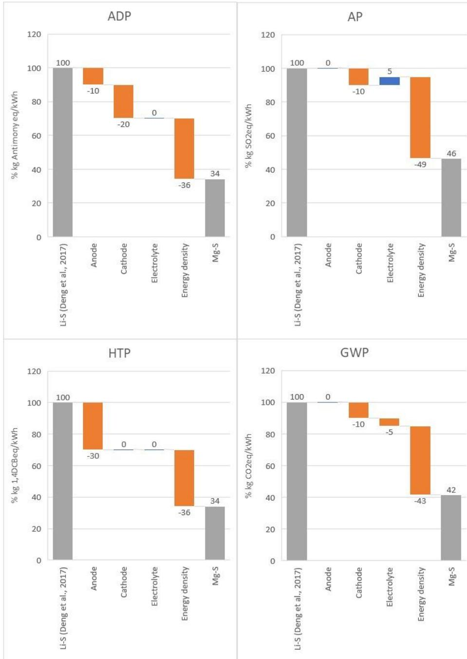
**Figure 18 :** Assessed environmental profile of the future Mg-S battery compared to Li-S reference battery.
